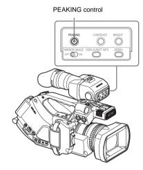
The color of the contours can be set with "Peaking" (page 123) of the VF SET menu. Turning the control back to its left stop position deactivates the peaking function.
